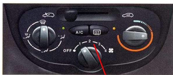
AC / Heater Control Panel
